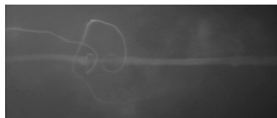
Fig. 11 30%-span ratio wing-tail configuration [b3 w4 t1 g40 r207] (rear views: left; side views: right); C_L = 0.615 .
